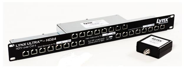
The Lynx Ultra is designed to deliver television (RF) on Cat 5/6 cable. It can distribute up to 804 digital channels or 268 HD channels over 100 meters of Cat 5 or Cat 6 cable. High frequency RF baluns in both the hub and end converters convert RF signals from a 75 ohm coaxial input signal to a 100 ohm UTP signal, and back again when the signal reaches the point of use. The product has bi-directional capabilities, and can be used in CATV, MATV, and SMATV applications.
