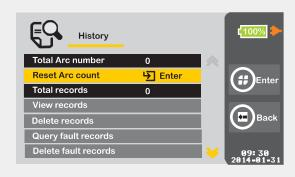
**Total Arc Number:** Electrodes arc times since the last record is eliminated.
