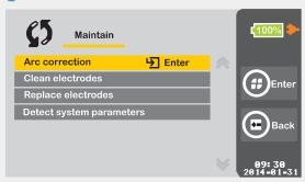
**Arc correction:** It performs an arc test and correction.
