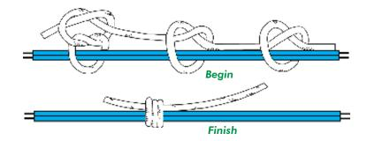
Once the knot is made, you simply make a series of lock stitches along the length of the bundle in equal intervals, again pulling tight as you go.
