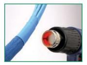
Gently apply heat from a heat gun, hair dryer or torch with an appropriate attachment. Keep the heat source far enough away so that hot metal or direct flame don't come in contact with the tubing, wires or sleeving. Move the heat around the bundle to prevent damaging the sleeving and to ensure that all areas of the tubing have been shrunk. Once cooled, your installation is complete.
